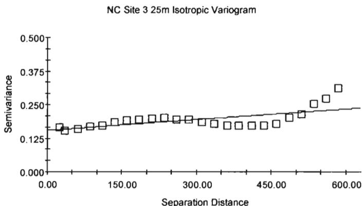
Spherical model ( $C_0 = 0.1539$ ;  $C_0 + C = 0.3468$ ;  $A_0 = 2110.00$ ;  $r^2 = 0.424$ ;
