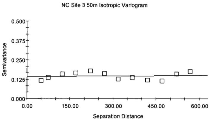
Linear model ( $C_0 = 0.1424$ ;  $C_0 + C = 0.1492$ ;  $A_0 = 568.33$ ;  $r^2 = 0.008$ ;
