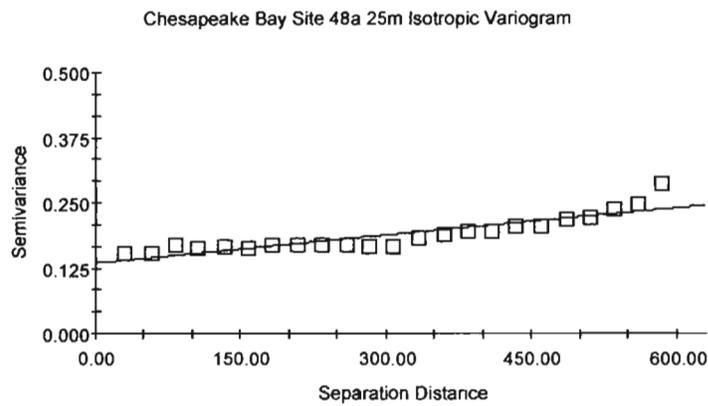
Spherical model ( $C_0 = 0.1343$ ;  $C_0 + C = 0.3876$ ;  $A_0 = 2110.00$ ;  $r^2 = 0.793$ ;  $RSS = 5.281E-03$ )
