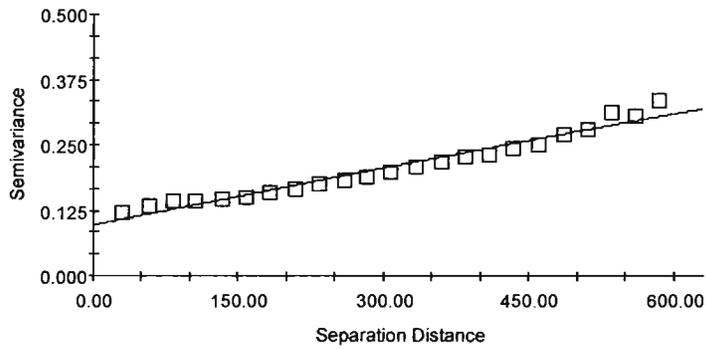
Spherical model ( $C_0 = 0.0970$ ;  $C_0 + C = 0.5600$ ;  $A_0 = 1899.00$ ;  $r^2 = 0.959$ ;  $RSS = 3.534E-03$ )
