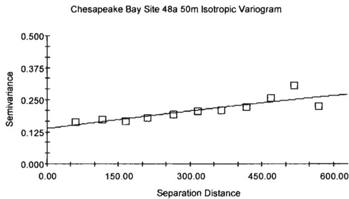
Spherical model ( $C_0 = 0.1376$ ;  $C_0 + C = 0.3272$ ;  $A_0 = 1222.00$ ;  $r^2 = 0.720$ ;  $RSS = 5.088E-03$ )
