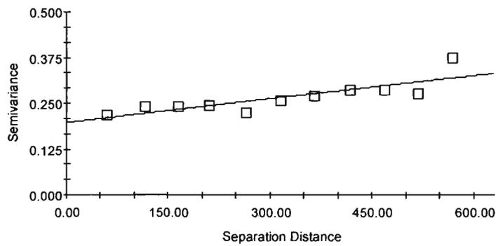
Spherical model ( $C_0 = 0.1971$ ;  $C_0 + C = 0.5062$ ;  $A_0 = 2110.00$ ;  $r^2 = 0.699$ ;
