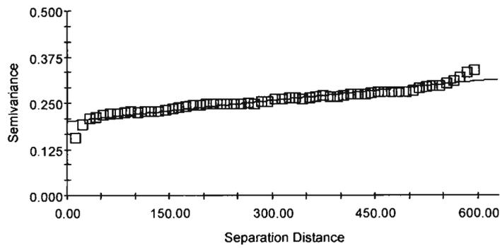
Spherical model ( $C_0 = 0.2002$ ;  $C_0 + C = 0.4014$ ;  $A_0 = 1591.00$ ;  $r^2 = 0.909$ ;
