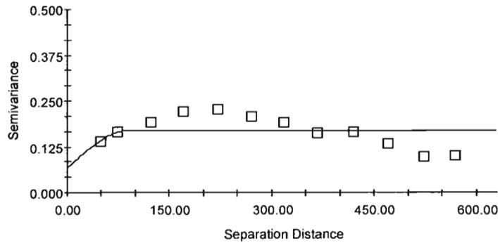
Spherical model ( $C_0 = 0.0664$ ;  $C_0 + C = 0.1698$ ;  $A_0 = 91.00$ ;  $r_2 = 0.037$ ;  $RSS = 0.0198$ )
