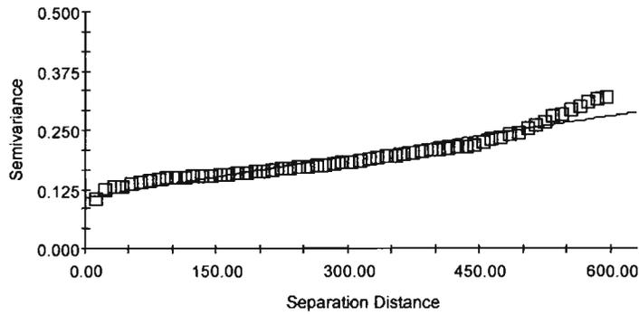
Spherical model ( $C_0 = 0.1070$ ;  $C_0 + C = 0.5220$ ;  $A_0 = 2110.00$ ;  $r^2 = 0.914$ ;  $RSS = 0.0134$ )
