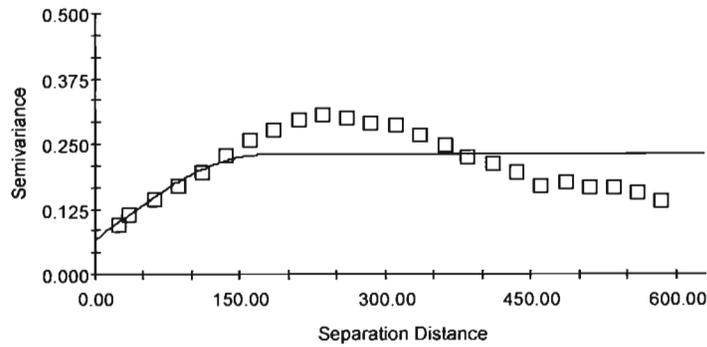
Spherical model ( $C_0 = 0.0656$ ;  $C_0 + C = 0.2292$ ;  $A_0 = 174.00$ ;  $r_2 = 0.381$ ;  $RSS = 0.0574$ )
