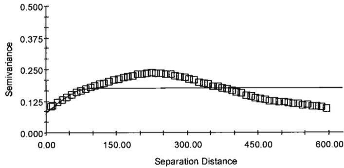
Spherical model ( $C_0 = 0.0770$ ;  $C_0 + C = 0.1740$ ;  $A_0 = 92.00$ ;  $r_2 = 0.120$ ;  $RSS = 0.108$ )
