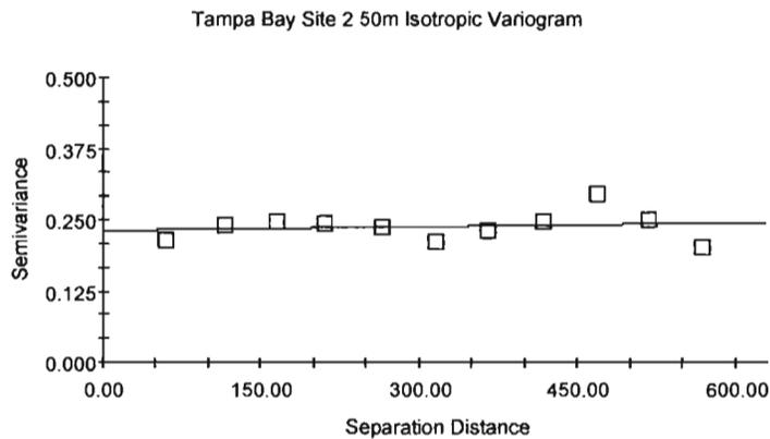
Linear model ( $C_0 = 0.2310$ ;  $C_0 + C = 0.2435$ ;  $A_0 = 568.33$ ;  $r^2 = 0.021$ ;
