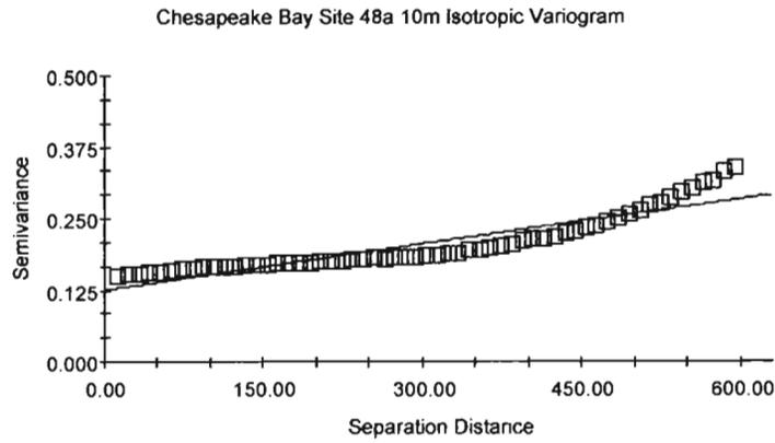
Spherical model ( $C_0 = 0.1250$ ;  $C_0 + C = 0.5060$ ;  $A_0 = 2110.00$ ;  $r^2 = 0.837$ ;  $RSS = 0.0238$ )
