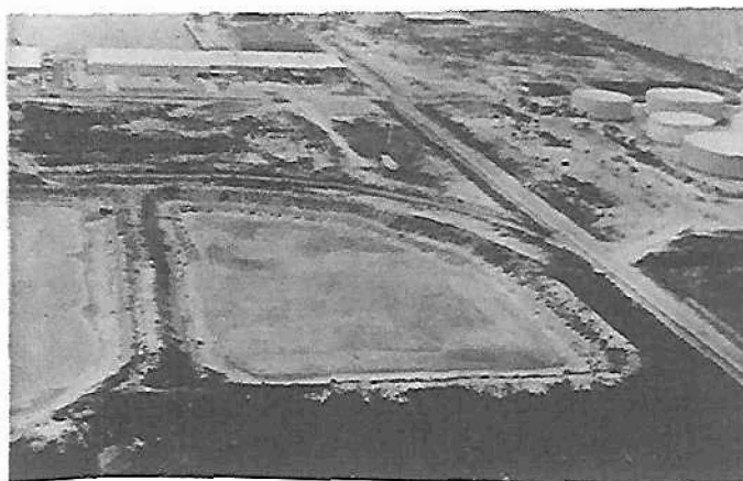
Figure 12. Diked upland disposal site for maintenance dredged material at Port Manatee, October 1976.
