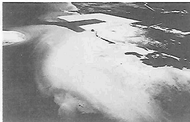
Figure 4. Dredging at Port Manatee, Lower Tampa Bay, June 1970. The channel creation and filling for the port is complete. Excess fill has been placed in the Redfish Creek mangrove forest, totally destroying it, and additional fill can be seen smothering the offshore seagrass meadows. No permits were issued for this work.
